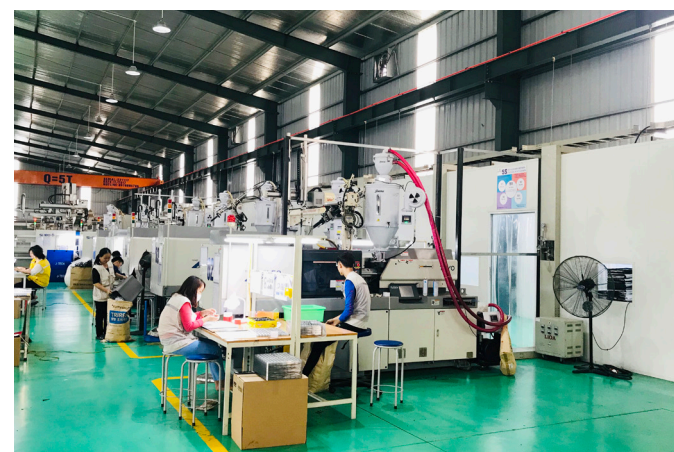
Injection Machine line
